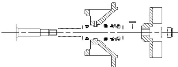
All gaskets should be replaced by new ones before assembly. Make sure PTFE and fiber based gaskets are not bent or broken when handled and installed.
