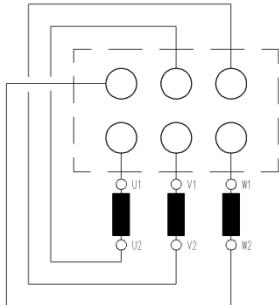
To change motor direction of rotation reverse two phases on wiring terminals. Connection of earthing terminal is mandatory.
