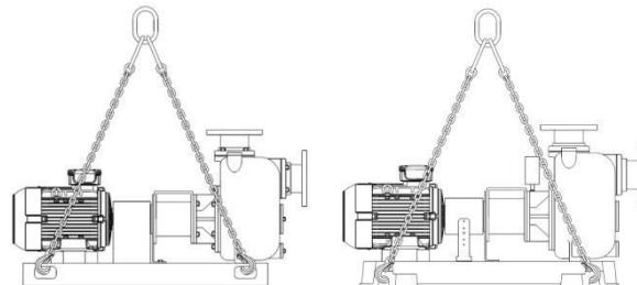
Lifting a bareshaft pump :
