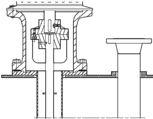
**VTM** : a bearing unit designed with ampli dimensioned ball bearing is placed between motor and matting flange. This design allows a length of more than 1920 mm under base plate. Ball bearings are lubricated by grease and shaft coupling is semi-elastic type.
