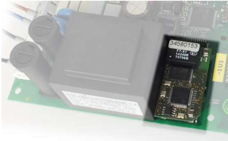
The Option plugs into the 32 Pin socket of SC-PCB. The The cut corner has to show away from the current transformer.
