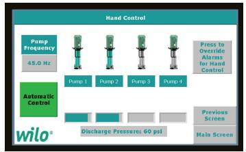
Once the pumps are switched from "Automatic Control" to "Hand Control", the screen will change; most noticeably, the green, "Automatic Control" button" will now read "Hand Control On".
