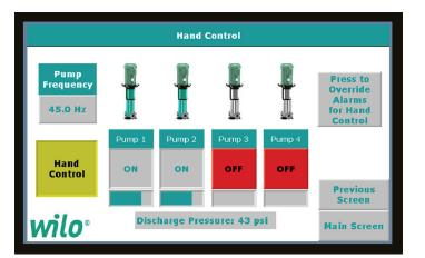
This mode allows the pumps to be turned on at a set frequency for manual control of the pump. Once you change a pump from off to on, a warning sign will pop-up on the display that informs you that if the frequency is set too high, damage can occur to either the pump or the components of the system. You can press the "override alarms for hand control" in order to bypass this warning.
