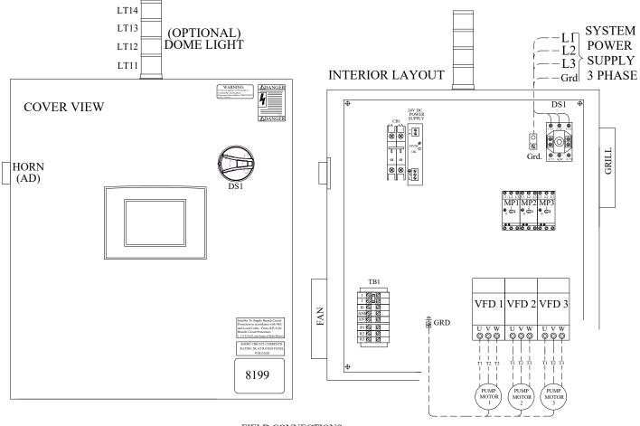
FIELD CONNECTIONS CONNECT EACH WIRE TO MATCHING NUMBER ON TERMINAL BLOCKS
