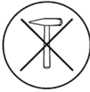
Fig. 6 Using a hammer for installation is not allowed
