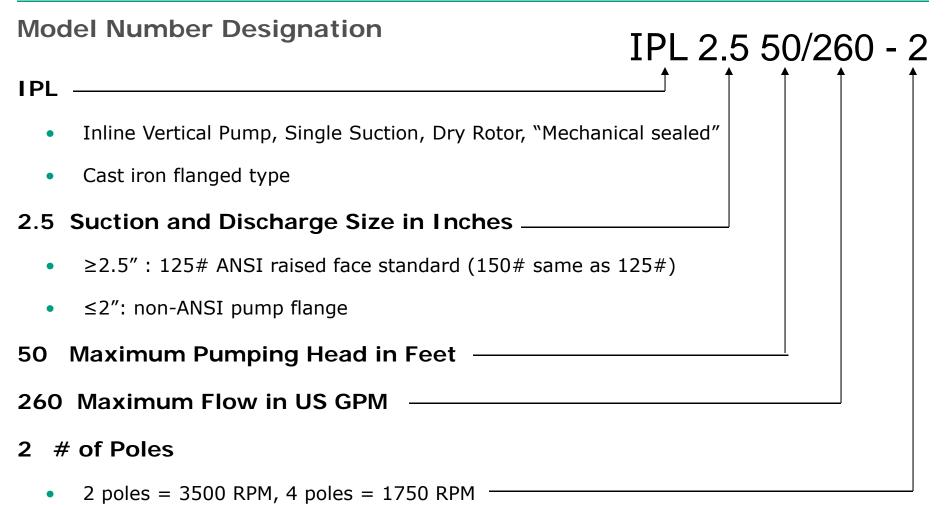
Note: Complete units include motor HP, motor enclosure, # poles (RPM), frame size, phase and voltage
