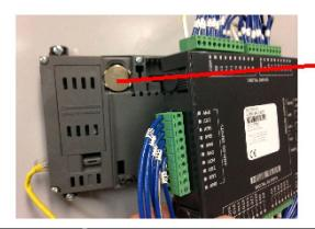
The battery is behind the I/O module. Slide the battery cover up to expose.
