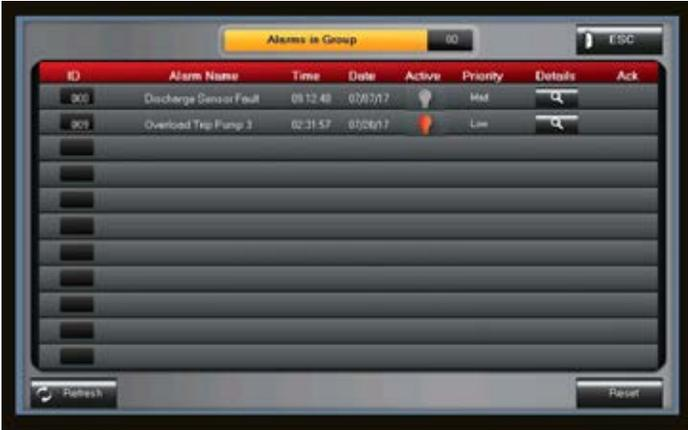
Hit the ESC button three times to return to the main screen.
