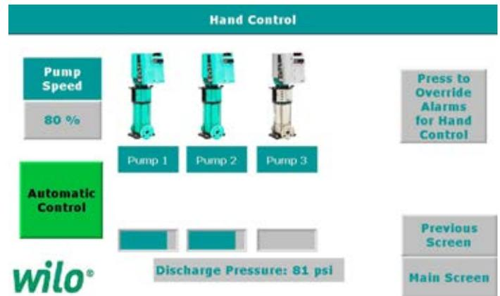
This mode allows the pumps to be turned on at a set frequency for manual control of the pump. Once you change a pump from off to on, a warning sign will pop-up on the display that informs you that if the frequency is set too high, damage can occur to either the pump or the components of the system. You can press the "override alarms for hand control" in order to bypass this warning.
