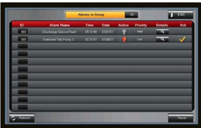
The check mark indicates that the alarm is acknowledged. The red light indicates the alarm is currently active, and the grey light means that the alarm has cleared, but has not yet been acknowledged. Default value is that alarms do not require acknowledgement to reset, except for the pipe burst alarm.
