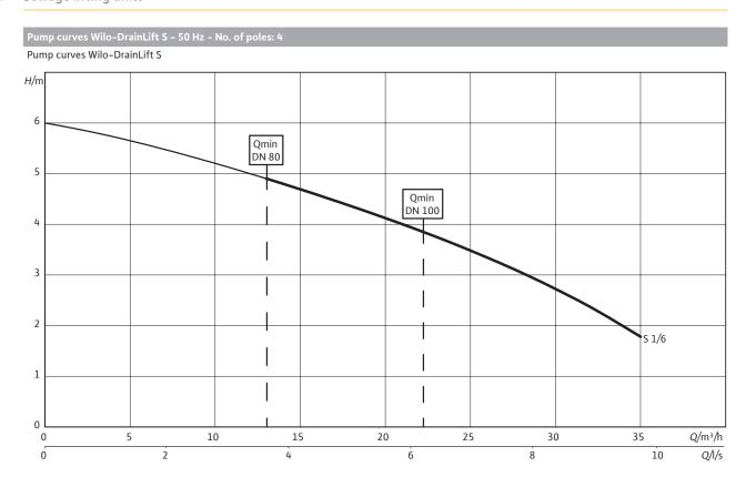
According to EN 12056-4, 6.1, flow velocity (in the pressure pipe) must be kept between 0.7 and 2.3 m/s. The stated  $Q_{min}$  values apply to the inside diameter of single-walled steel pipes.
